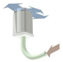
The VM FlexVac converts any IQAir filtration device into a wall-mounted, self-contained extraction system that allows to capture fumes, dust and vapours at the source.
